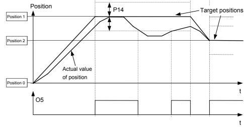
For purposes of clarity a poor loop setting is shown here.
